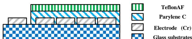
Fig.2 Cross section of the EWOD device
