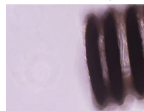
Fig.5 Myotube on micro coil. Dimension from left to right is 1 mm.
