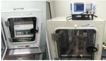
Fig. 8: Centrifuge (left) and vibration (right) in incubator.
