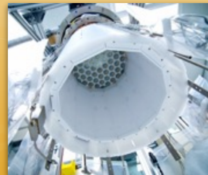
Active region defined by PTFE reflectors (high reflectivity >97%) - high light collection)
