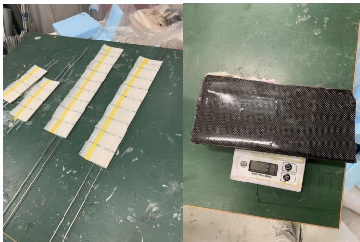
Fig21.(左図)翼心材 (右図)積層後の翼
